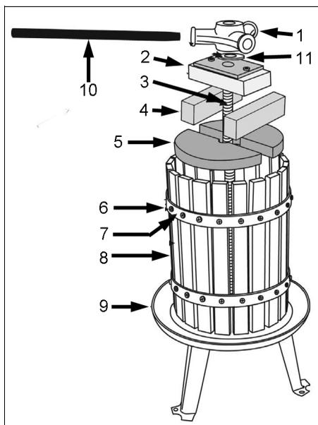
the pressure plate (2) on top of these, as shown in the illustration. Place a container beneath the outlet spout in the base (9) ready to collect the juice.
